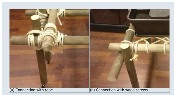
Figure 43: Connections tested for the prototype
