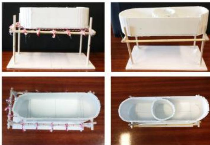
Figure 29: Carboard model (single module)
