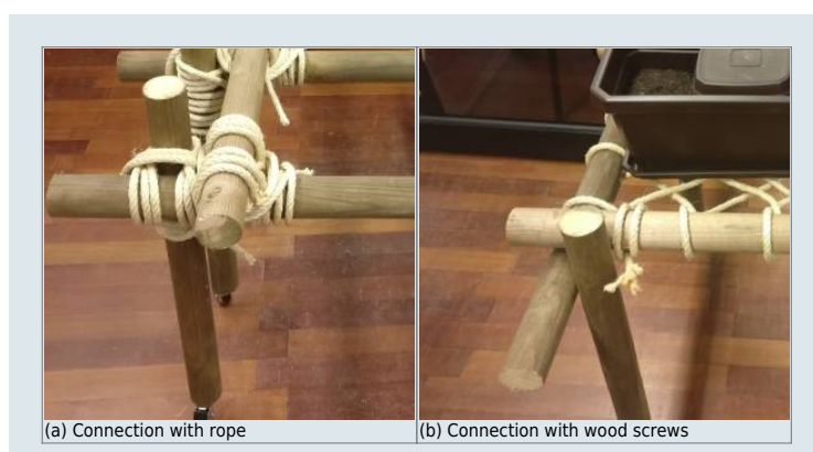
Figure 43: Connections tested for the prototype
